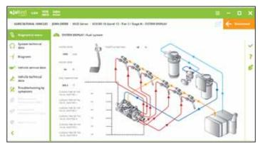
Software shows model specific information for finding and clearing fault codes.
