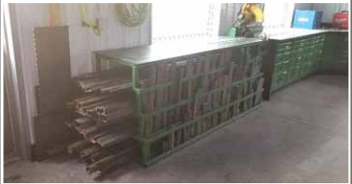
Welding table has metal storage below, a cut-off saw and is 10-ft. long.
