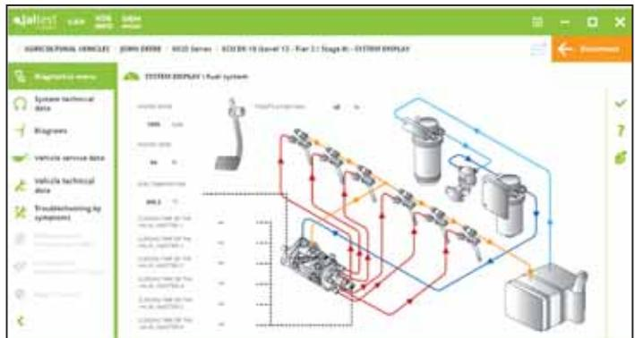
Software shows model specific information for finding and clearing fault codes.
