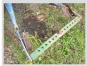
Tom Dufrense, Grant, Minn.: "The drawbar on my Ford utility tractor spins freely in the hitch pins and was a constant annoyance when hooking up trailers or other equipment. So I came up with a pair of 'stops' to hold it in place.
