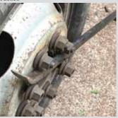
"When tightening wheel studs on truck or car tires, you can use a pry bar to hold the wheel in place. Just insert it across the wheel between the studs and rest the end on the ground."
