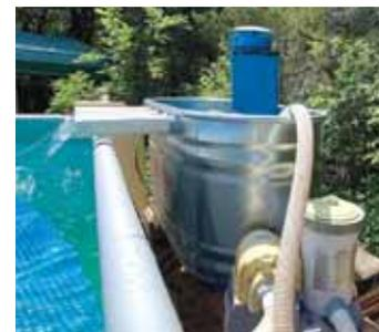
**A propane-powered livestock tank heater warms the water.**
