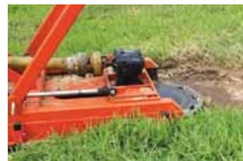
Cutting wheel is moved into trees with hydraulics and is fitted with carbide cutting teeth.
