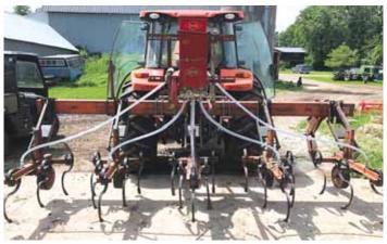
Barlage added a gravity fed interseeder to his cultivator, allowing him to drop cover seed on freshly tilled soil.
