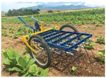
The 4-ft. wide Tiny Treffler harrow can be pulled by hand, horse, or tractor. The pressure can be adjusted from 7 oz. to 11 lbs. depending on crop needs.
