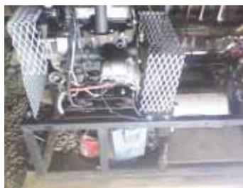
A 3-cyl. diesel engine belt-drives 10,000-watt generator to keep batteries charged. Expanded metal safety shields cover the belts.
