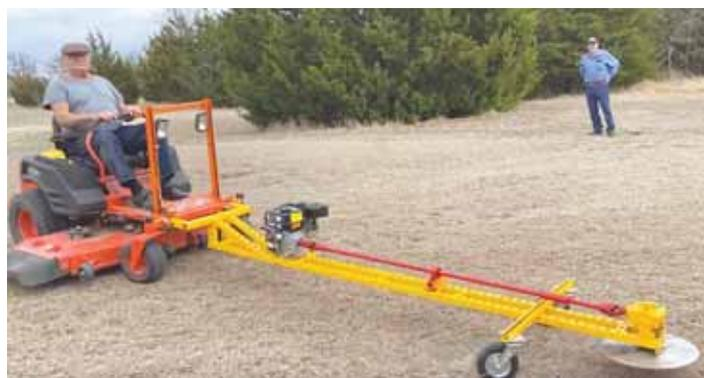
20-in. saw mounted on 10-ft. lengths of construction strut keep tree cutter a safe distance from the mower.
