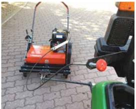
Modifications to the dethatcher include caster wheels for maneuverability. a hitch for towing behind a mower with an extended throttle cable. and a turnbuckle for height adjustments.
