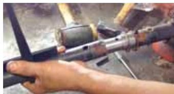
company website make it even easier. The first step is to remove reel fingers to either side of the bearing to verify the pipe style, should the original reel have been replaced previously. Combine models with their OEM pipe reels in place can be checked against the kit "fit" list.
