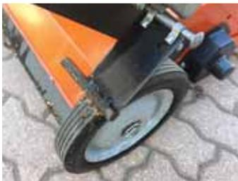
Small scrapers that rest on the rear wheels and are pinned to brackets he mounted to the dethatcher.
