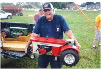
The RC pullers build their own tractors using engines from weed wackers and snowblower tires. Servos from model airplanes control the throttle and steering.
