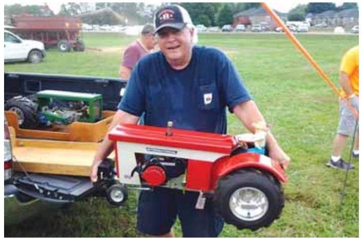
The RC pullers build their own tractors using engines from weed wackers and snowblower tires. Servos from model airplanes control the throttle and steering.
