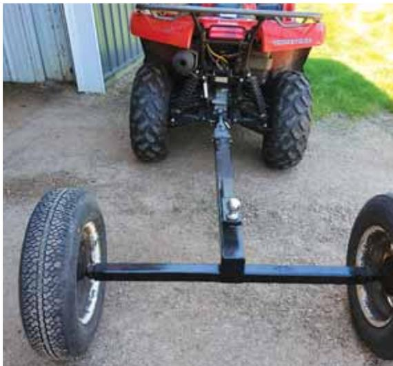
Rick Schmitz used an old boat trailer to make a dolly that can handle over 1,000 lbs. of tongue weight. The compact dolly makes it easy to move trailers with his ATV.
