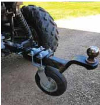
Another idea he had was to bolt a wheel to a receiver hitch to help keep the back end up when towing.
