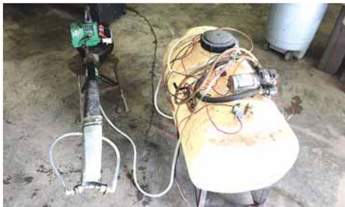
Wadel's mist sprayer uses a lawn sprayer tank, pump, and flood spray tips powered by a leaf blower fitted with an extension. It can spray up to 25 ft. high.
