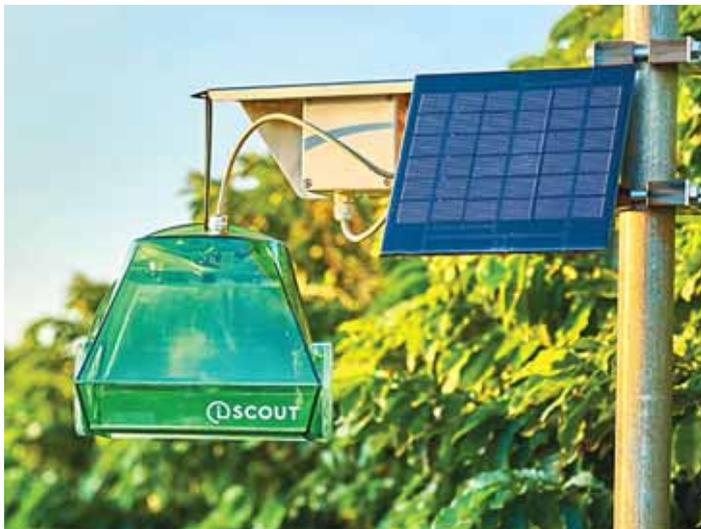
As the traps capture insects, the cameras inside show infestations in real time so producers can quickly determine how and when to react.
