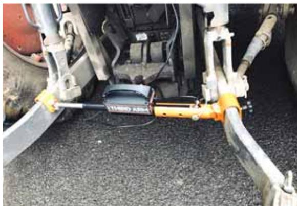
The Third Arm can be mechanically adjusted nearly 6 in. to match different category hitches.
