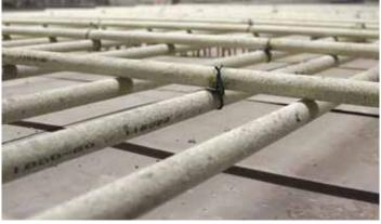
Pultrall fiberglass rebar doesn't react to salt, chemicals, or alkaline in concrete. It has an expected life of more than 100 years in concrete slabs.
