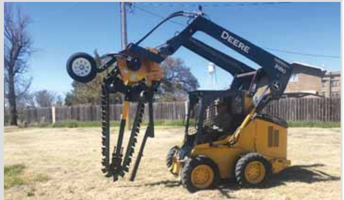
Hydraulic trench attachment digs a trench 48 in. deep and 6 in. wide or more with extensions.
