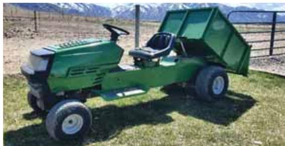
Johnson extended the frame of his riding mower and added a 3 by 3 1/2 ft. dump bed for chore work.
