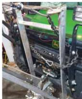
To adjust the pole out farther, Faulkner runs short chains between the hooks and the cable loops on the frame.
