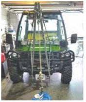
The Gin Pole uprights are welded to a base plate that bolts to the snowplow frame. The base plate has 2 by 2-in. steel tubing that slide into the Gator front receiver hitch.
