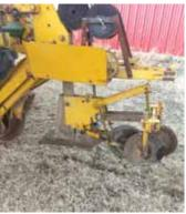
Jacob removed the seed hopper and plates, then mounted a free turning wire reel. He replaced the seed tube with a stainless steel tube similar to a fertilizer tube.
