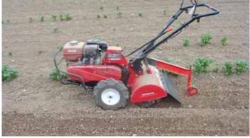
The drag bar on the rear tine tiller was replaced with a 5-in. wheel to keep mulch from building up under the bar.
