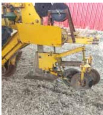
**Jacob removed the seed hopper and plates, then mounted a free turning wire reel. He replaced the seed tube with a stainless steel tube similar to a fertilizer tube.**
