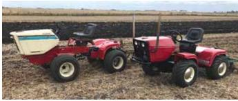
Bruggeman figures it takes 5 tractors to make one quad. A 682 supplied the hood and 1 transmission. The 1864 supplied its power steering, frame, and the second transmission.
