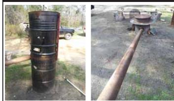
Gary Mull smokes plain cheese using a firepit, 10-ft. long pipe, and two 55 gal. drums. The long pipe keeps smoke cool so it doesn't melt the cheese.
