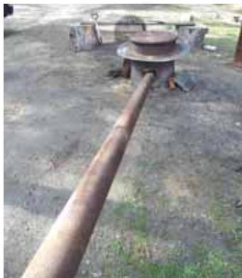
Gary Mull smokes plain cheese using a firepit, 10-ft. long pipe, and two 55 gal. drums. The long pipe keeps smoke cool so it doesn't melt the cheese.
