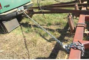
Log chain attached to an implement helps to reduce sway while driving on highway.
