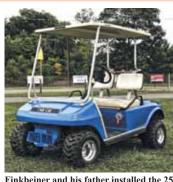
Finkbeiner and his father installed the 25 cu. in. 2-cyl. diesel engine in the cart and modified the drive system to work with the cart's transaxle.
