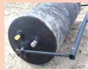
Large washers were used for the diameter of the flue. The axle matches the hole in the washers, and a short piece of pvc acts as a bushing for the roller.
