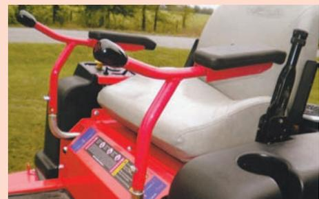
The operator can also control the machine by pushing a pulley on the arm rests alongside the seat.
