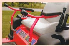
The operator can also control the machine by pushing a pulley on the arm rests alongside the seat.
