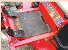
Pushing on toe portion of foot pedal controls forward movement, and pushing down on heel portion controls reverse. Pushing down farther either way controls speed.
