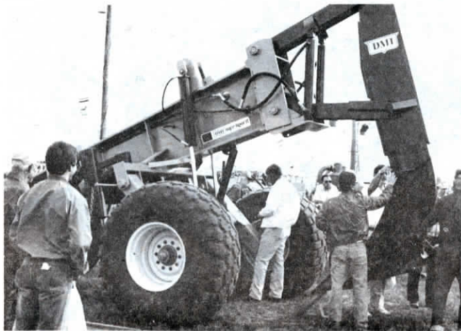
The big 3,200-lb. parabolic shank requires 60,000 to 100,000 pounds of drawbar pull.
