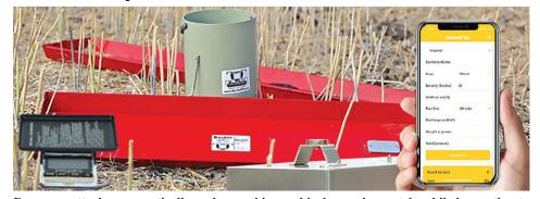
Drop pan attaches magnetically under combine and is dropped remotely while harvesting to collect a sample of chaff and straw. A downloadable app shows bu. per acre grain loss.
