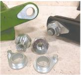
According to Burgei, S.I. Distributing, Spencerville, Ohio, bushings are a common problem Flange bushing has a small builtworn parallel linkage arms and with today's planters. "In the
