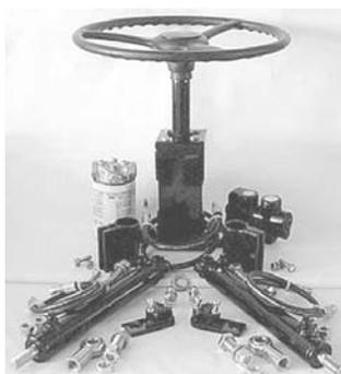
This JPS Power Steering Kit would fit on a Ford tractor. Steering units for other models will differ as far as the components.
