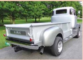
He used 16-ga. sheet metal to build the floor and bed sides for the 11-ft. bed. Note the deep well custom wheels.
