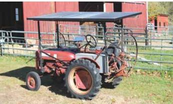
This Farmall Cub Lo-Boy has 3 solar panels mounted on top. Its engine was replaced with a 10 hp. DC motor powered by six 12-volt batteries.
