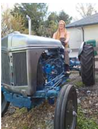
Courtney Koster replaced the worn-out 4-cyl. engine in her 1940 Ford 9N with a Ford Falcon in-line, 6-cyl. engine. "I learned to weld from my dad as a teen, and he and grandpa were mechanics, so the work comes naturally to me," she says.
