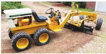
Frank Smith used a pair of vintage Cub Cadet garden tractors to build this 13-ft. long motor grader. It's powered by a 12 hp., Kohler air-cooled engine.
