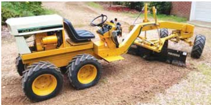
Frank Smith used a pair of vintage Cub Cadet garden tractors to build this 13-ft. long motor grader. It's powered by a 12 hp., Kohler air-cooled engine.
