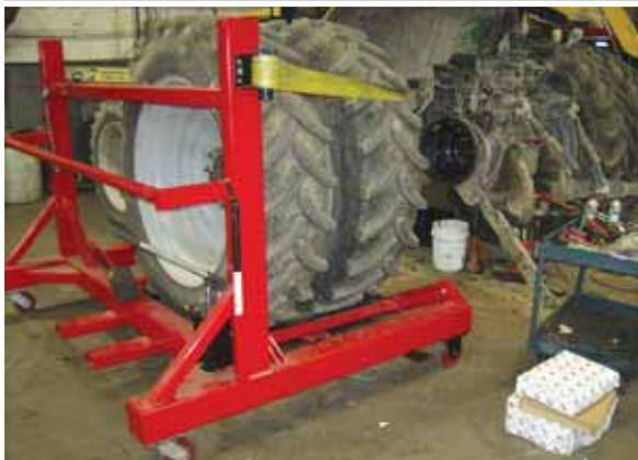
**Tire cart design makes it easy to raise, secure, and reposition wheels safely and quickly.**
