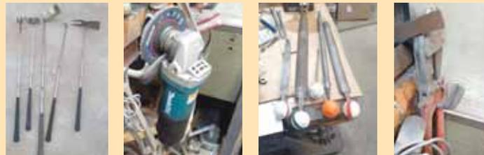
**Shipman’s uses for old golf equipment include replacing club heads with small garden tools, turning an old pitching wedge into a grinder holder, using golf balls as file handles, and using heads on irons as hooks.**
