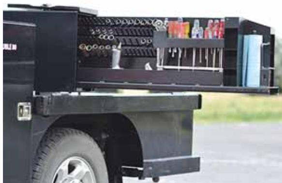
**I-80 toolbox comes with an 80-in. long insert that holds all your tools and can be rolled out from either end of toolbox.**
