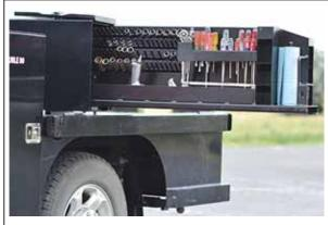
toolbox comes with an 80-in. long insert that holds all your tools and can be rolled out from either end of toolbox.
