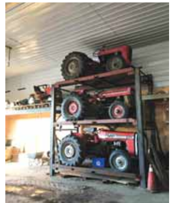
Suurdt built a rack using 12-in. I-beams and 2 by 6-in. square tubing to hold his 6 Massey Ferguson tractors. He moves them with a 5,000-lb. forklift.
