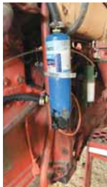
Kunau screwed a 120-volt water heater element into bottom of propane tank. Cold coolant flows into bottom of tank as warmed coolant flows out the top.
