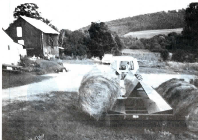
The A-frame runs down the middle of the hauler-feeder and raises up 16 in. to push bales off either side of wagon. The 20-ft. long rig handles five 4-ft. dia. bales per side.
