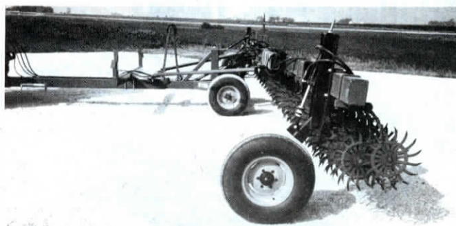
Converting a 3-pt. hoe to pull-type lets you take a wider swath with a smaller tractor.
