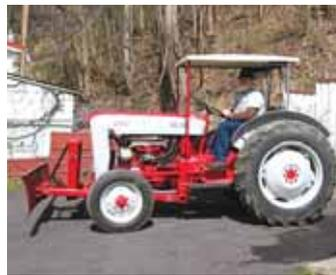
Mike Wingler uses the 3-pt. hitch on his tractor to lift front-mounted implements, with help from a subframe, scissors lift, and boom arms.
