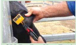
A battery and solar panel are integrated into the reusable ear tag to power the GPS transmitter. It sends out location signals to area antennas every 2 hours.
