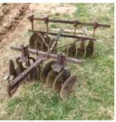
This 3-ft.tandem disk has a universal joint in the middle, allowing disk's rear gang to follow directly behind front gang on turns.
