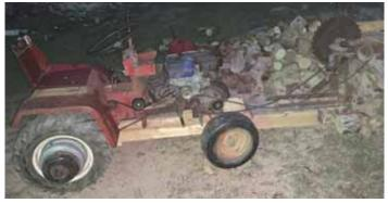
The 18-in. blade on this home-built sawmill is belt-driven off the same shaft that drives WheelHorse's belly-mounted mower.
