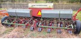
Cut-apart grain drill mounts on back of Forde's 8-row, 20-in. CIH Cyclo planter. He uses the setup to seed oats in rows alongside corn and soybeans.
