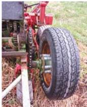
When Forde lowers planter to the ground, its wheels press against grain drill tires to drive the seed meters.
