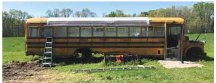
Seals cut out the sheet metal between vertical ribs on bus, then bolted 2 by 4’s on the sides and top to attach greenhouse plastic.
