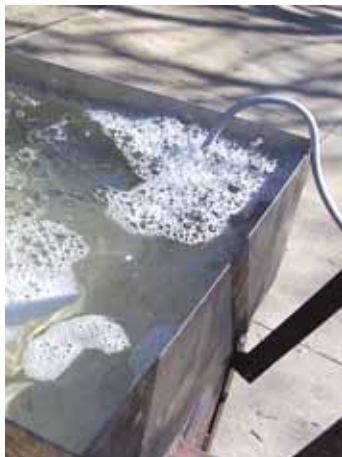
Compressed air is heated before being used to aerate syrup. Aeration speeds up evaporation.
