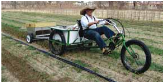
Boyd's custom 28-speed bike can haul up to 300-lb. loads. It can pull a spreader, or be used to cultivate fields with its oversized tires.
