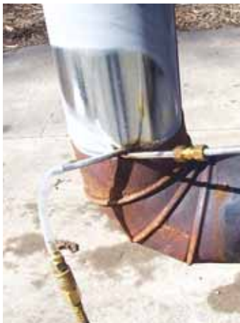
Compressed air is heated before being used to aerate syrup. Aeration speeds up evaporation.
