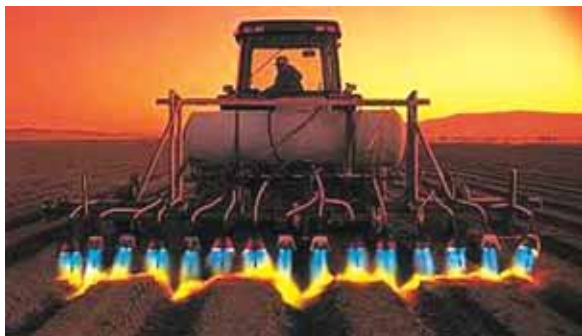
Red Drag Vegetable Bed Flamer can be used before planting to sterilize the seedbed.
