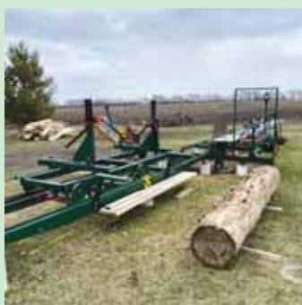
Carriage on antique sawmill rides back and forth, delivering logs to a 48-in. dia. blade. Solar-powered kiln dries cut wood fast.
