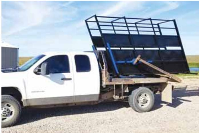
The EZ Load Chute can be picked up by the arms on a common bale bed and hauled to where it is needed.
