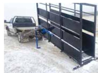
Chute's legs are adjustable to match the height of your truck or trailer bed.
