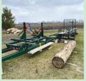
Carriage on antique sawmill rides back and forth, delivering logs to a 48-in. dia. blade. Solar-powered kiln dries cut wood fast.
