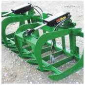
Charles Murphy, Piereeto, Ind.: "My sons and I clean out a lot of fence rows and also cut firewood, and for such jobs we use an 84-in. stone bucket with dual cylinder root grapple attachments that we bought from Skid Steer Attachment Depot in Huntsville. Alabama (www.skidsteerattachmentdepot. com; ph 256 975-8641). These grapples work great for cleaning out brush and holding up the logs we cut for firewood."
