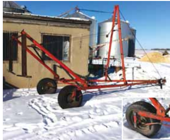
The Johnsons used the hinged auger support brace at rear of the running gear to carry the bale. They moved the vertical, fixed A-frame with its winch to a midway point on the running gear frame.
