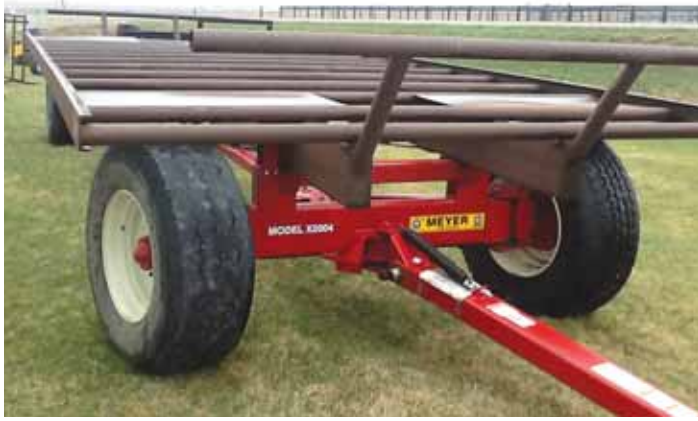
Frederick uses thick-wall oil well pipe to construct the bed on his bale carriers. The biggest units can hold up to 14 round bales.
