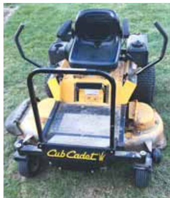
Hand Hold Bar bolts onto front of mower. "You just put your hand on it, step on the deck, and grab the steering handles," says inventor Dick Lewis.
