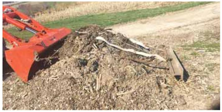
**Steel railroad tie chained to loader bucket holds the load together, allowing Tschetter to haul big loads of loose material.**
