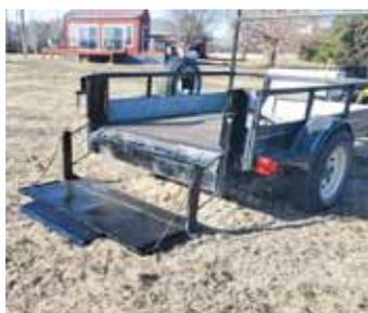
**Cervený built a 4 by 8-ft. trailer and added an old Tommy Gate lift and 12-volt deep-cycle battery to make trailer easy to load.**
