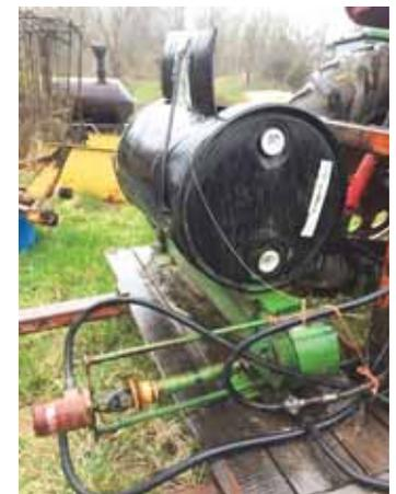
**Hempel used a 55-gal. plastic barrel and the grain conveyor off an old combine to build this 3-pt. mounted cube feeder.**
